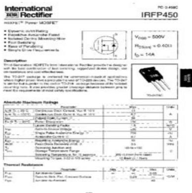
The image shows the datasheet for the IRFP450 MOSFET. It includes the International Rectifier logo, the part number IRFP450, and various technical specifications. Key parameters listed include V<sub>DS</sub> = 500V, R<sub>DS(on)</sub> = 0.40Ω, and I<sub>D</sub> = 14A. The datasheet also features a pinout diagram, a photograph of the component, and tables for Absolute Maximum Ratings and Thermal Resistance.
