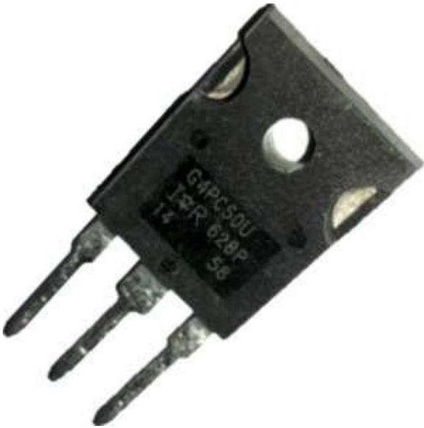
IRG4PC50U: IGBT 600V 55A Ultrafast Speed IGBT
