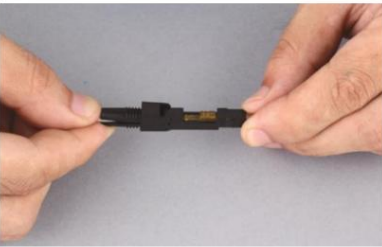
10.Close the gland for fixing drop cable
