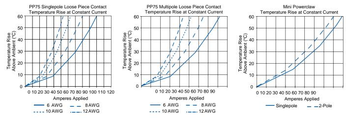
NOTE: Powerclaw charts are based on #8 AWG equivalent copper foil on board side, mated to #6 AWG conductor on wire side.
