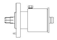
Reducer, 50 ohm, 1-5/8-inch to type N female, gas tight with pressure port, includes inner connector and flange hardware kit. Formerly part number 2261A.
