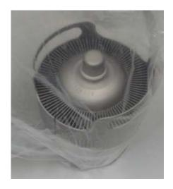
The 4CX3500A is a compact tetrode designed to be used in VHF power amplifier service. It features a type of internal structure which results in high RF operating efficiency up to 220 MHz. This tube is also recommended for use as a VHF TV linear amplifier.
